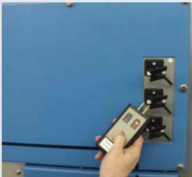
Self-testing of DEHNcap/A voltage indicator.
