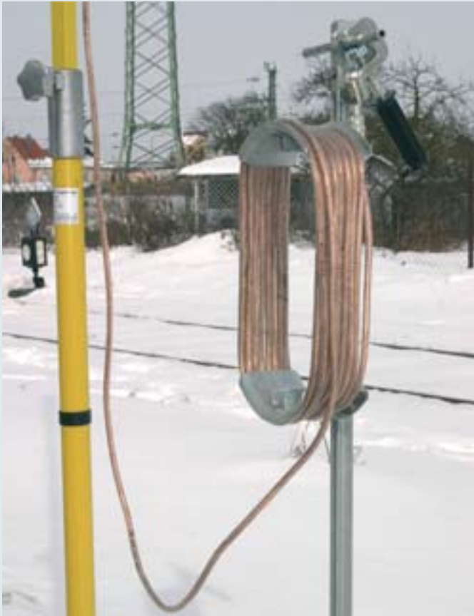
Earth spike with coiled earthing cable.
