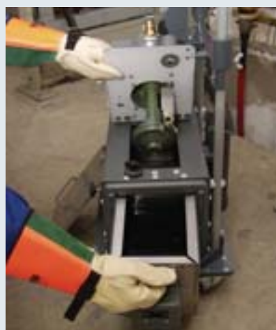
After pulling out the conveying pump from the HT mass, the oil reservoir can be removed for refilling.
