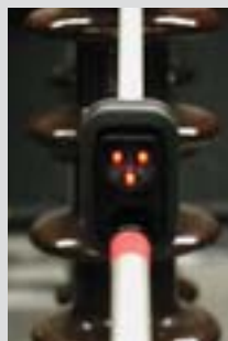
Three flashing LEDs staggered at 120° improve the visibility of the indication "voltage present".
