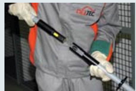
Attaching the extension handle type HV STK to the insulating rod type IS PHE STK.
