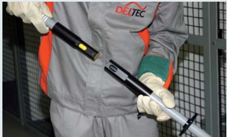
Attaching handle extension type HV STK to insulating rod type IS PHE STK.
