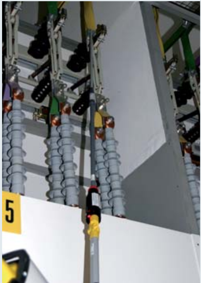
PHE III voltage detector with attached test probe.
