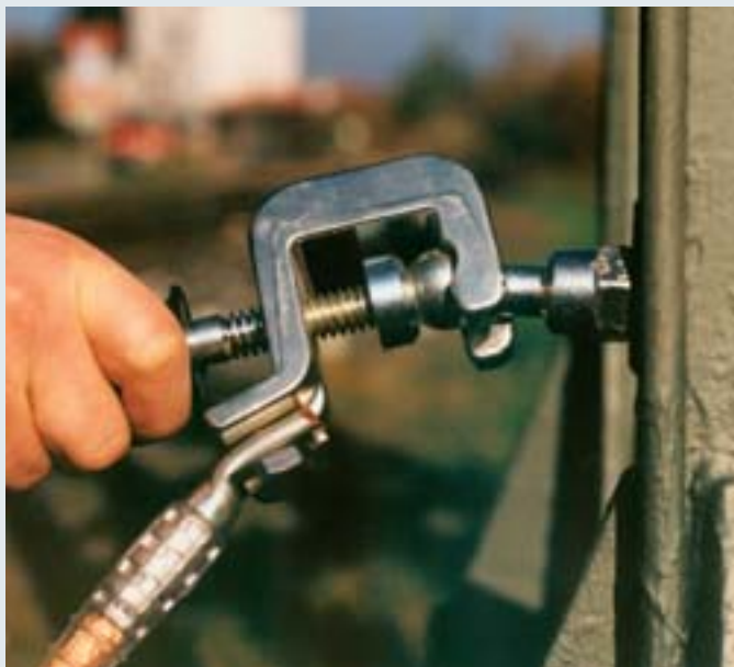
Universal earthing clamp with insulated handle connected to a fixed ball point.
