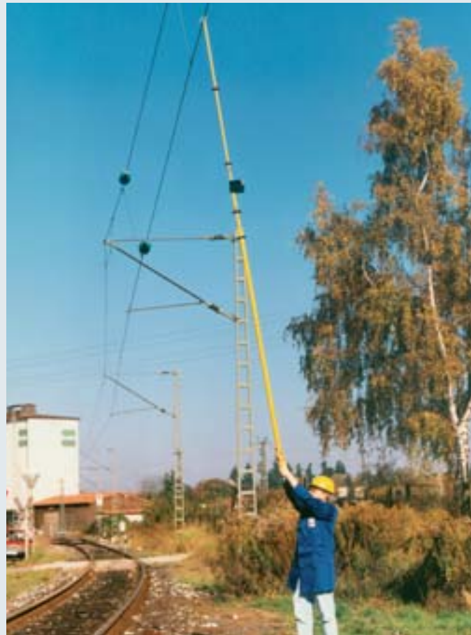
PHE Voltage Detector with visual indicator used on an overhead contact line of the German national railways.
