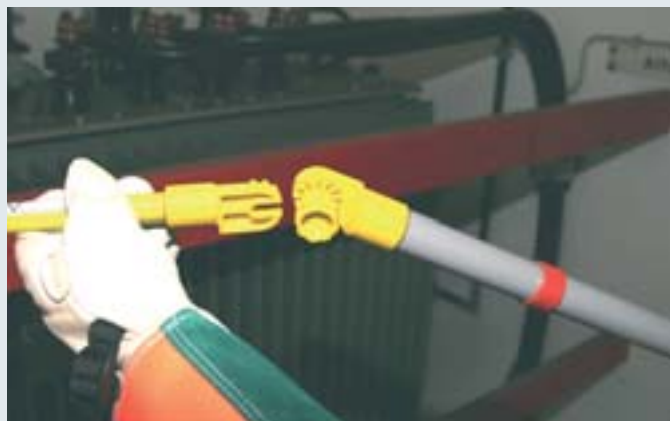
The universal gear coupling allows for quick exchange of the operating head and extensions.
