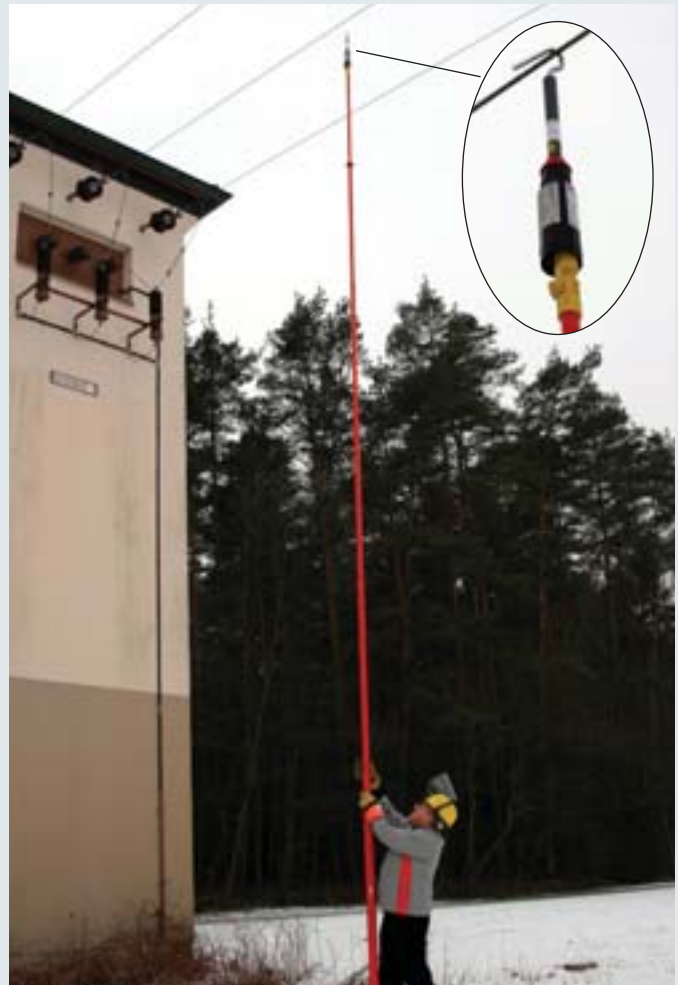
Telescopic insulating rod for PHE III electronic indicator.
