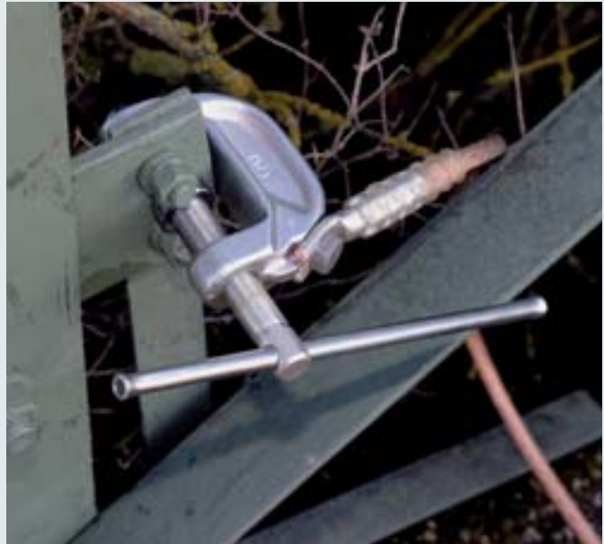
Earth milling clamp used for coated steel masts.
