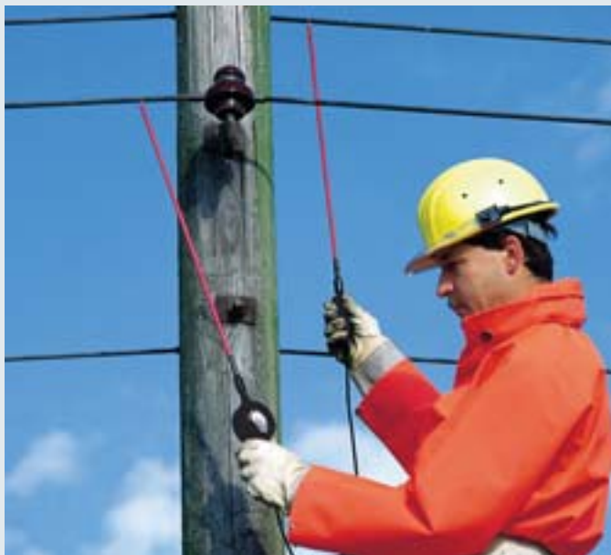
Two-pole SPN voltage detector used with extension prods in overhead lines.
