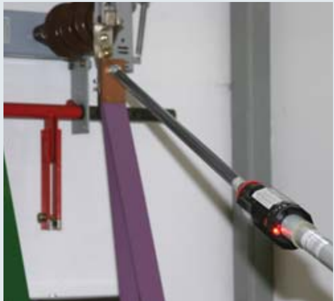
PHE III Voltage Detector with visual and acoustic indicator used on an indoor switchgear installation.
